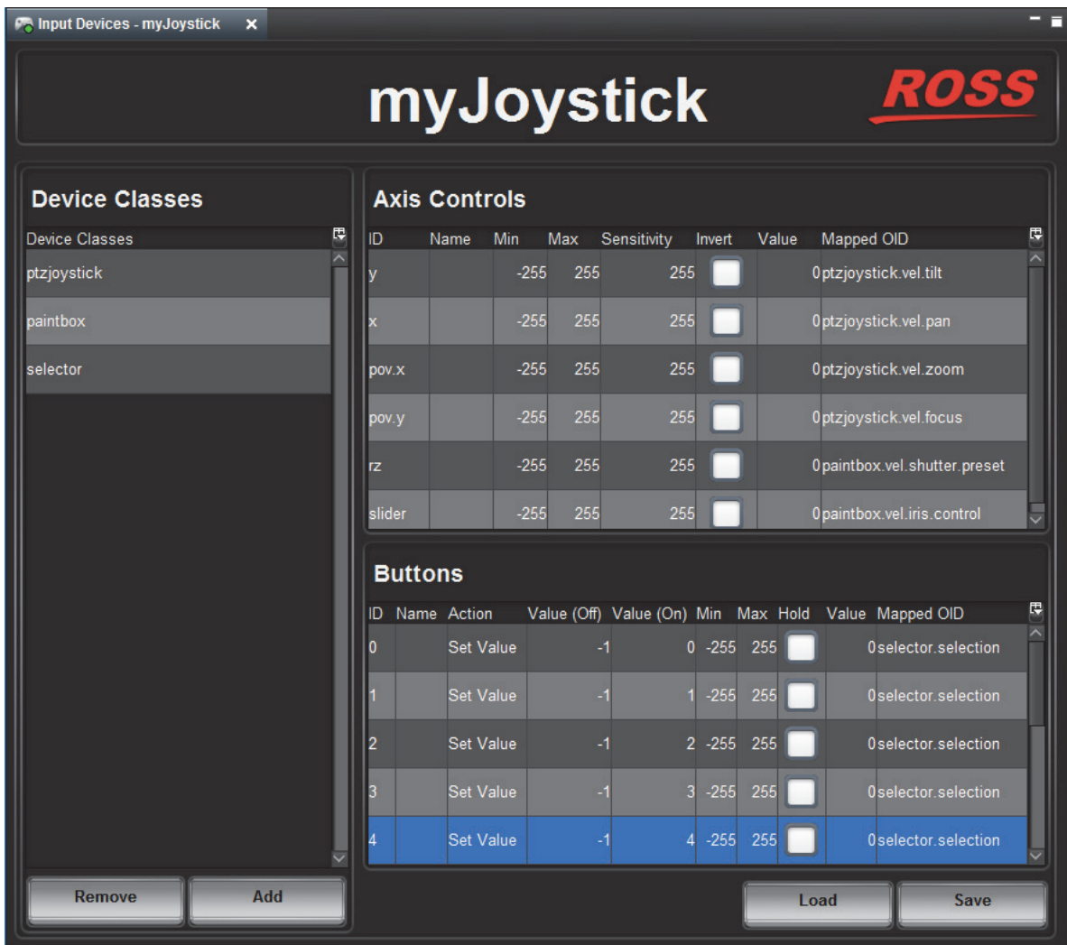
Figure 5.3 - Mapping USB Controller Data to PIVOTCam Control Panel Parameter OIDs
